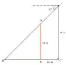
From the diagram, we can see angle  $\angle ABC = 63^{\circ}$  because of alternate angles. From this we can work out the length of BE.
